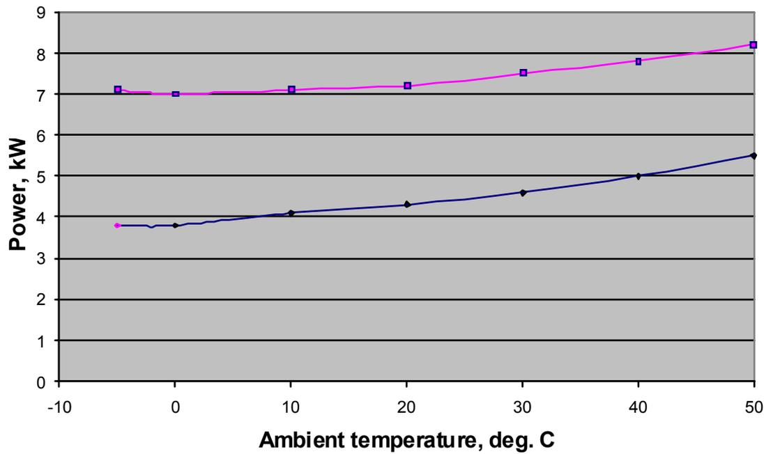
**Figure 1.** Power draw range for refrigerated containers of various designs at steady temperature conditions, 50 and 60 Hz operation, -1 to +13 °C cargo temperatures.
