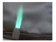
Figure 6 - Flame Halide Test Showing Chlorine
