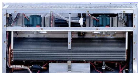
Figure 6 - Carrier Everfresh Air Compressor
