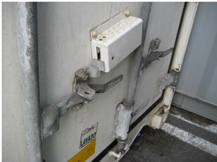
Figure 11 - Carrier Everfresh Automatic Door Lock
