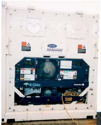
Figure 5 - Carrier Everfresh System
